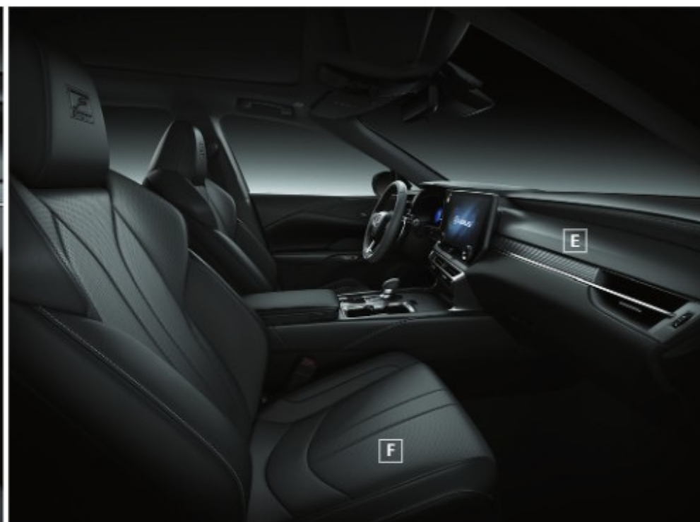
F SPORT Performance/F SPORT features A_Dimpled leather steering wheel with paddle shifters / B_Dimpled leather shift knob / C_12.3-inch full LCD meter / D_Aluminum sport pedals and footrest / E_Real aluminum ornamentation / F_Leather sport seats F SPORT exclusive features G_Emblem / H_Scuff plate
